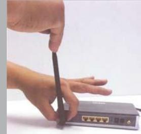
DO NOT rotate the entire antenna around the unit during installation
