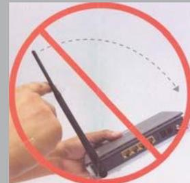
Improper installation of the antenna can cause the connector to snap from the unit
